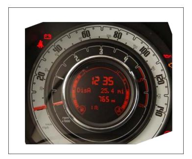
The speedometer is assembled with two dials on top of each other. The outer dial has two axes—mph and km/h. The inner dial is the rpm meter, which has a different scale and style. Another uncommon feature is that the body parts of both dials are hidden underneath; only the top needle parts are displayed. In the center of the gauge is an LED screen showing journey information. Using all these unique appearances, Highcharts provides enough flexibility to assemble a chart that looks very similar.
