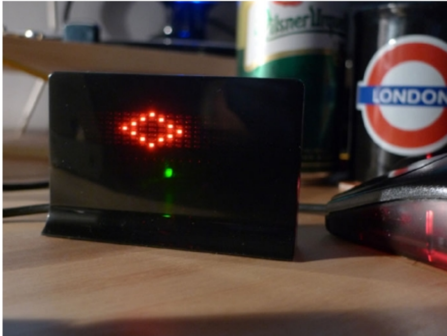
Figure 5.20 LED message board blinking with a red eye to tell you about a failed build
