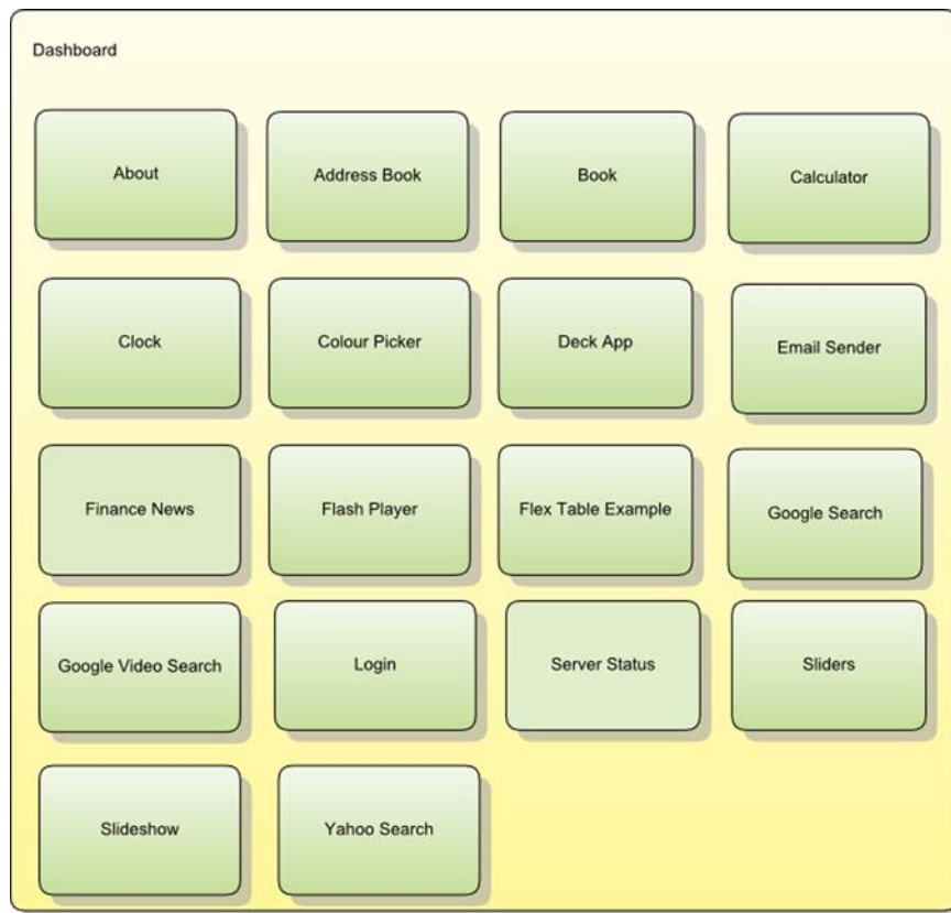
Figure 9.2 The module structure that will be used in developing the complete Dashboard application. The component application modules will all be inherited by the main Dashboard module.
