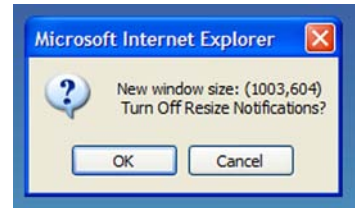
Figure 6.13 The result of resizing the browser window with a WindowResizeListener set up to display the new size
