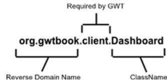
Figure 2.6 Breakdown of a GWT fully qualified Java class name for your application. This is standard Java syntax, but GWT requires that your user interface code always be under a subpackage called client . (We cover other special subpackage names such as server and rebind at various points later in this book.)
