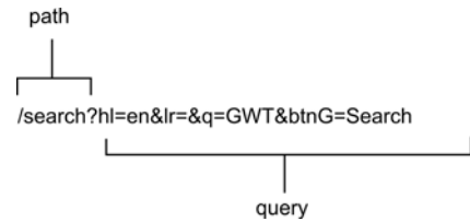
Figure 12.1 The anatomy of a URL, used to reference some piece of content on a server
