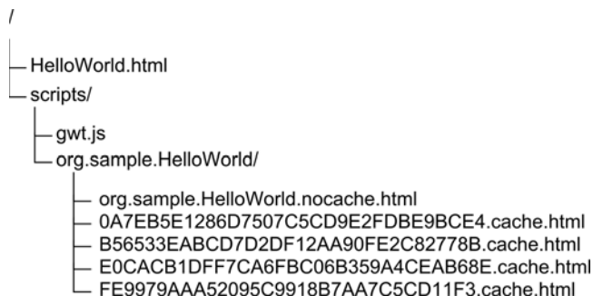
Figure 16.6 An example of a reorganized GWT application that uses a directory to hold scripts and modules
