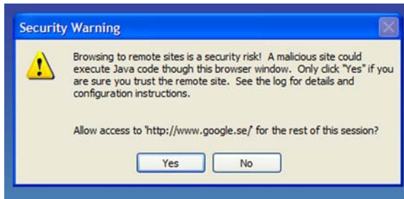
Figure 3.9 The security warning that GWT hosted mode raises if the user or code tries to navigate to a URL that isn't specifically included on the whitelist
