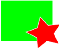
Figure 4.25 PNG image transparency problem in IE 5.5: a white halo around the star using the GWT Image widget
