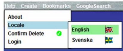
Figure 4.10 Examining the Dashboard's menu system and showing off the two new MenuItem widgets built in this chapter. The English and Swedish locale MenuItem s are instances of the TwoComponentMenuItem , and the Confirm Delete MenuItem is an instance of the ToggleMenuItem (it's shown in the ON state).
