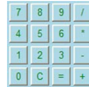
Figure 4.18 A range of Button widgets set out to form the keypad of the Calculator Dashboard application
