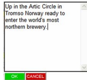
Figure 7.12 Buttons moved underneath the text area purely by defining this in the associated CSS
