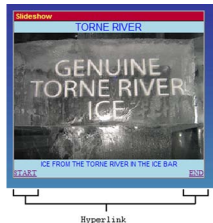
Figure 4.6 Two Hyperlink widgets ( Start and End ) in action at the bottom of the Slideshow Dashboard application
