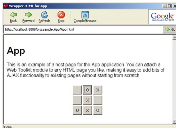
Figure 1.6 Tic-Tac-Toe GWT application running in the hosted-mode browser. This is how your screen should appear if you're following along with the code.
