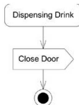
Figure 8-14. Transition-oriented view of a signal being dispatched
