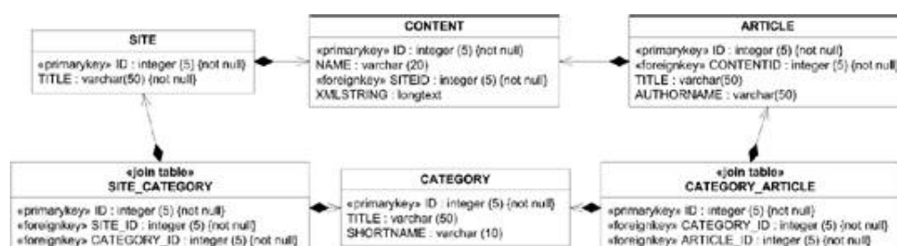
Figure 2-39. An example database schema using a class diagram
