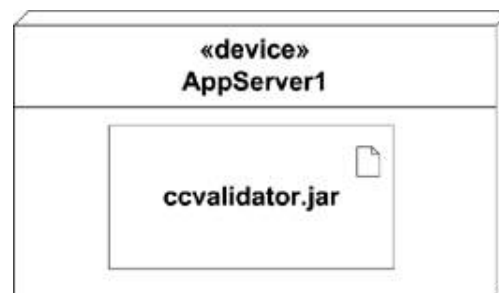
Figure 6-13. An artifact deployed to a device
