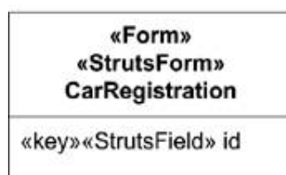
Figure 11-4. A class and an attribute, with two stereotypes each
