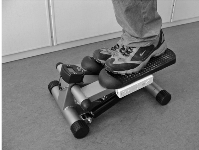
Figure 9.15 Wii Remote attached to consumer fitness device.
