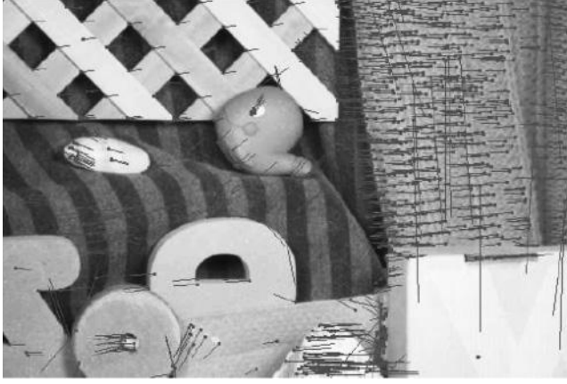
Figure 4.64 Sparse Lucas–Kanade flow vectors. (From [41]. Copyright © 2008 IEEE.)
