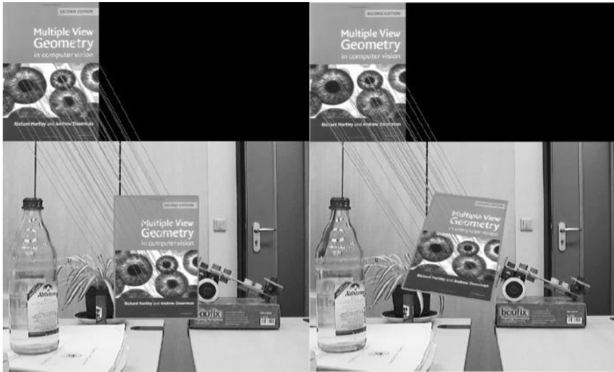
Figure 6.12 Three-dimensional pose estimation with invariant keypoints: GPU-based implementation.
