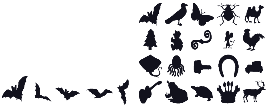
Figure 4.19 Matching shapes with Zernike moments. The shape of a bat undergoing variations due to the viewpoint ( left ) is matched successfully to the top-left shape on the right. (From [94].)
