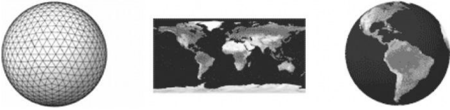
Figure 2.17 Texture image mapped onto a polygonal mesh.
