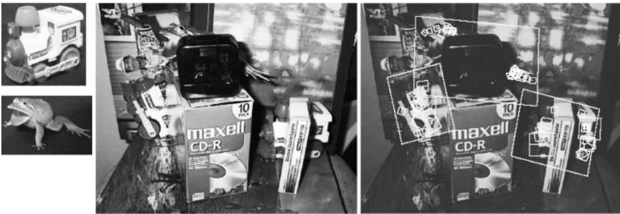
Figure 6.11 Model-based object detection with SIFT keypoints. Multiple instances of the train model are found even in the presence of occlusions. (From [106].)
