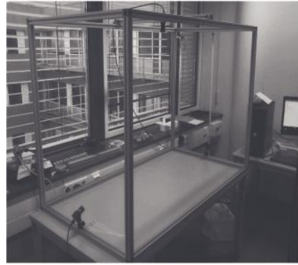
Figure 7.23 Multicamera setup for three-dimensional object tracking.
