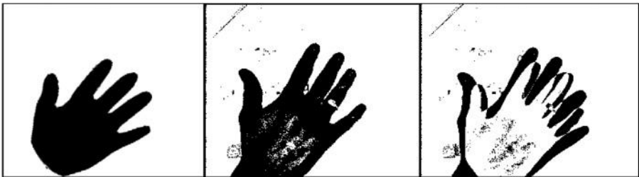
Figure 3.5 Example of pixel-level measurement. Left : expected object shadow; middle : foreground segmentation on the real image; right : residual image. (From [100].)
