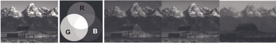
Figure 4.2 RGB color space decomposition. (From [24].) ( See insert for color representation of the figure. )
