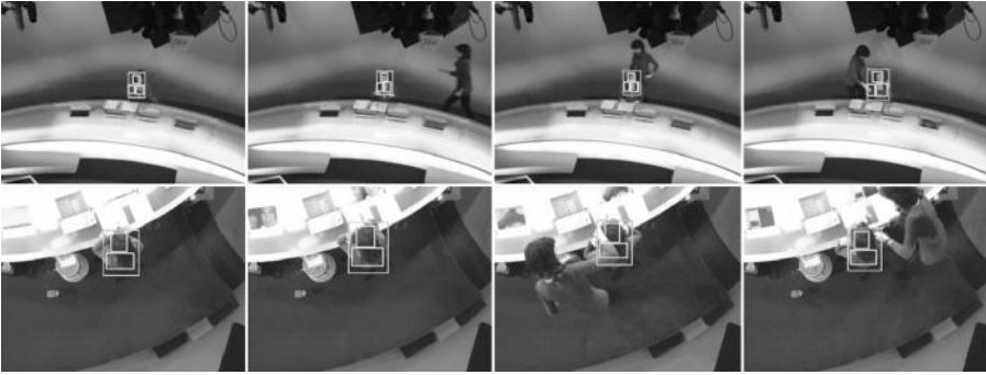
Figure 7.20 People tracking with a multipatch color histogram model. Top row : frontal camera frames; bottom row : overhead camera. (From [126,127]. Copyright © 2008 IEEE.)
