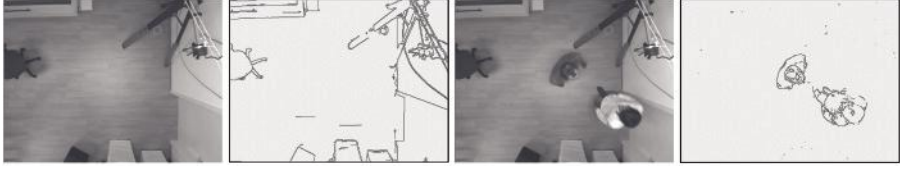
Figure 4.16 Subtraction of background edges using the Canny detector. Left to right: background model; background edges; current image; remaining edges after background subtraction.
