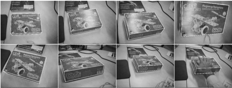
Figure 4.75 Mutual information for three-dimensional object tracking is a robust index with respect to light and shading variations as well as partial occlusion. (From [134].)
