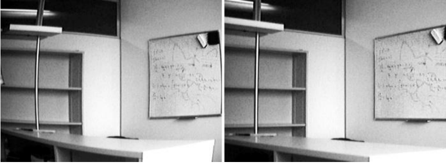
Figure 2.5 Left : image with radial distortion; right : corrected image, after estimating the distortion coefficients. (From [101].)
