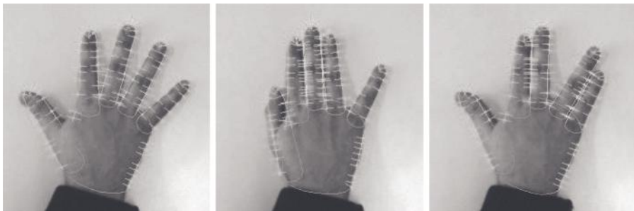
Figure 7.18 Monocular, articulated hand tracking with contour points, combining CCD and intensity edges. Sampled contour points and normals are shown. (From [132].)
