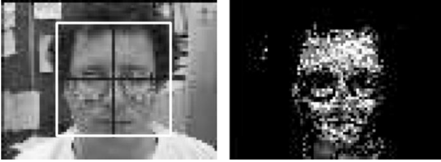
Figure 4.9 Back-projection of an image on the model color histogram. Left : original image and model; right : back-projection on the model histogram. (From [45].)
