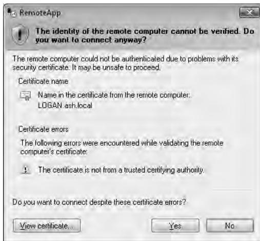
FIGURE 9-39 Avoid getting an error by adding the certificate containing the farm name to the RDP Tcp Properties General tab of RD Session Host Configuration.
