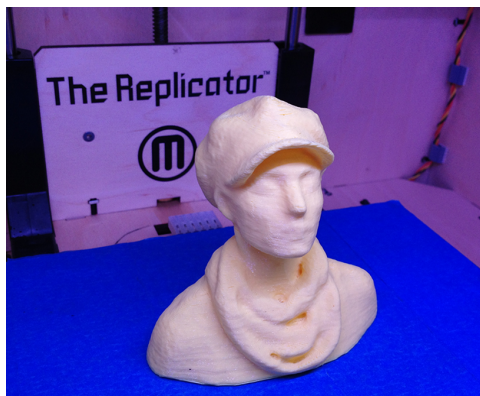
Figure 9-26. Final printed ReconstructMe scan
