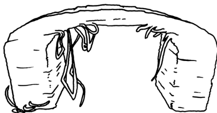
Figure 8-1. Overhangs can produce droopy and fluffy layers
