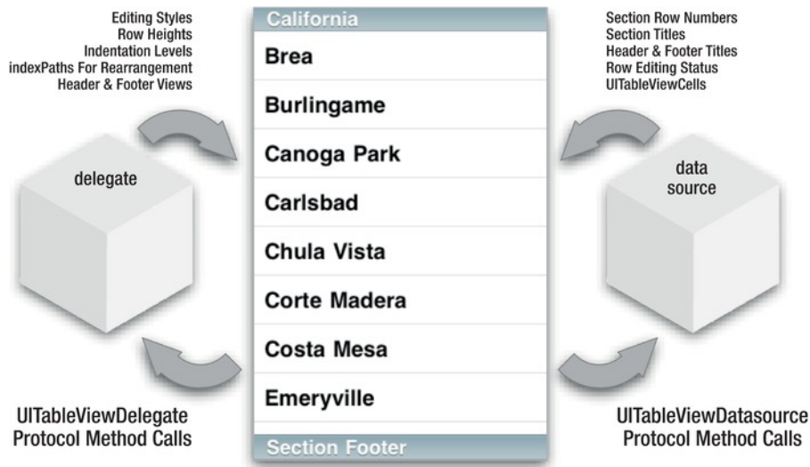
Figure 3-4. How the tableView interacts with its delegate and dataSource
