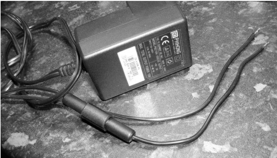
Figure 2-5. A repurposed 5 volt supply
