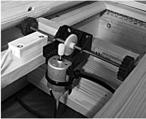
Figure 8-6. Panel drive assembly (with motor)
