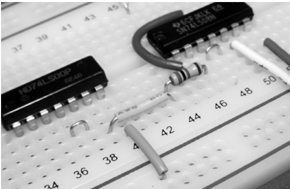
Figure C-9. Connecting the resistor via unused breadboard column 44
