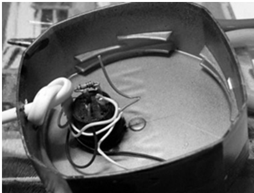
Figure 10-7. The coffee jar lid button mount
