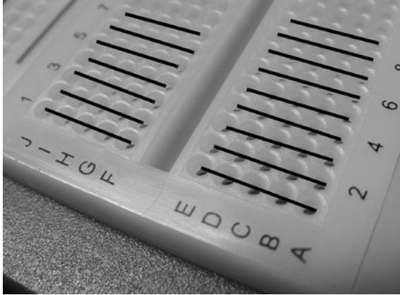
Figure C-2. Interconnected column holes
