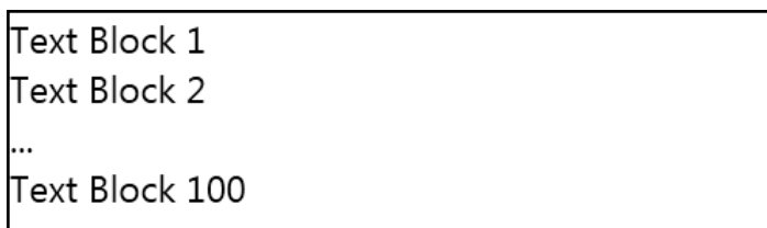
Figure 5-5. StackPanel with Vertical orientation
